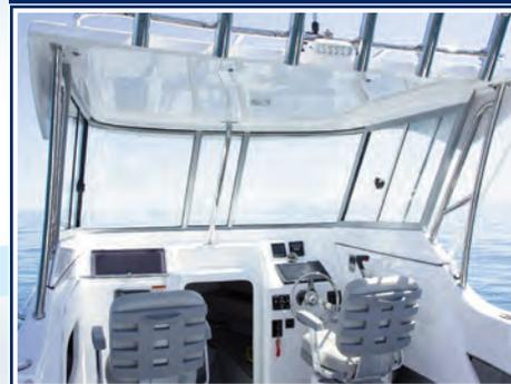
*Fully enclosed toughened glass hardtop, for the ultimate in weather protection*
